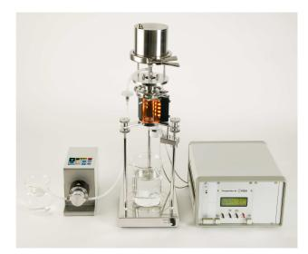
Continuous gear pump with digital magnetic coupled drive system and pump head with PEEK gears 85 up to 264 V, 47 up to 60 Hz, 60 W, 50 up to 5'000 rpm, 0.85 up to 85 ml/min.
